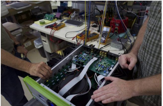
After the amps and preamps are assembled, they are taken to a room that is kept at the same temperature year around for break-in and biasing. This assures that the bias of every Pass amp that goes out is identical. All Pass amps are burned in by running power through them for three days.
